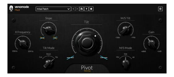
At its core, pivot is a tilt equalizer, meaning that you can adjust the amplitude of the spectrum like a seesaw. Move the big knob to the left and the low end becomes quieter as the high end becomes louder, and vice versa.
